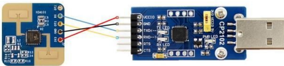
Figure 4-1 Connection between the HLK-LD2420 hardware and the USB-to-TTL serial adapter board
